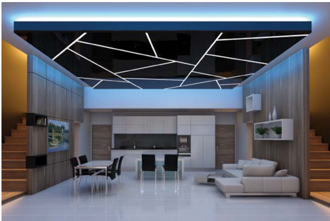
KEYLIGHT SYSTEM COMPRISES OF ALUMINUM PROFILE AL18, LED-SOURCE AND DIFFUSOR VEC-1 OR VEC-2
